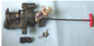
Figure E - Turn adjuster hex in the tighten direction to drive the piston all the way out of the bore.
