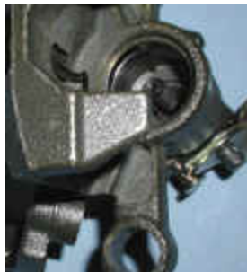
Figure G - With the piston and dust seal out of the way, we can see the piston seal in its groove at the mouth of the cylinder. Carefully remove piston seal with a pick.
