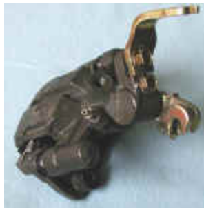
Figure B - Allen adjuster cover bolt below bracket. Bleed nipple and brake line port can be seen in this view.
