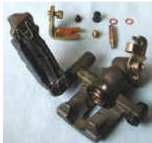
Figure C - Remove one slider pin, under cap, with 10mm wrench. Flip open to remove brake pads, w-clips, and brake pad slide clips.
