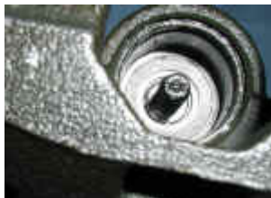
Figure G - With the piston and dust seal out of the way, we can see the piston seal in its groove at the mouth of the cylinder. Carefully remove piston seal with a pick.
