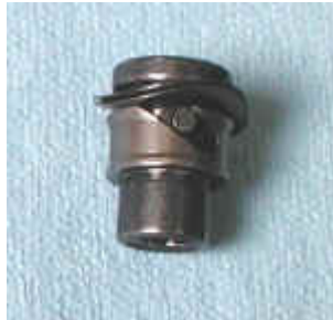
Figure P - Remove external c-clip and slid off toothed wheel.
