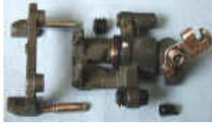
Figure D - Brake pads are set aside, this shows the orientation of the slider pins, boots, and caliper body.
