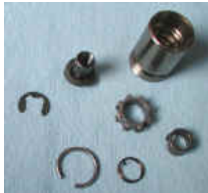
Figure Q - Collar with inclined slot lifts off completing disassembly. Wave washers are retained on hub by pressed in pin. We did not remove the pin as we were not certain it could be successfully reused. We have satisfied ourselves that there is nothing to replace here and fortunately nothing to wear out either.
